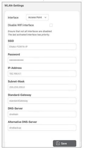
The WLAN and the LAN interface can each be deactivated. Otherwise both interfaces are active.
